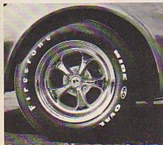
ABOVE—Keystone Rogues and Firestone F60's replace the stock slotted wheels and radials.
